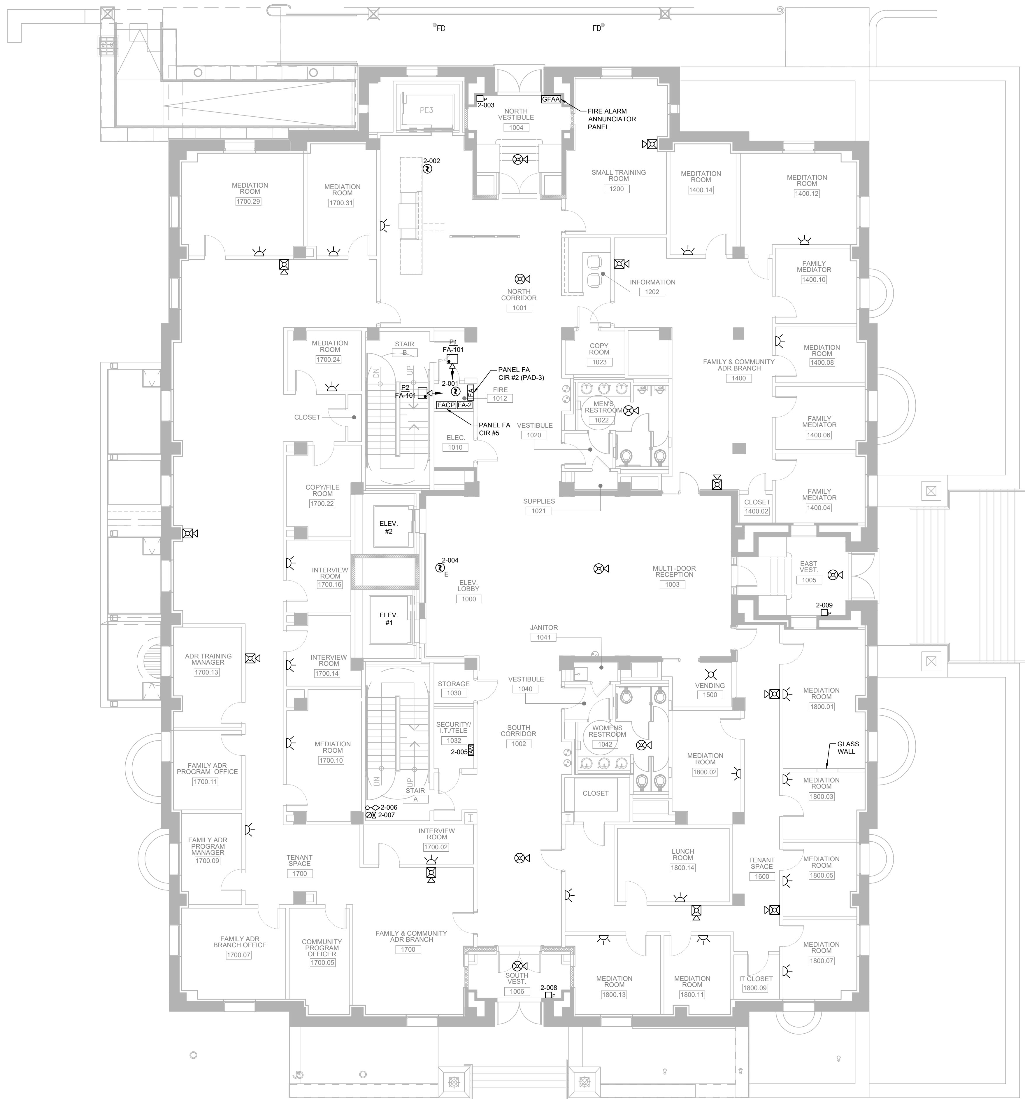
1 FIRE ALARM SYSTEM FIRST FLOOR PLAN SCALE: 1/8"=1'-0"
